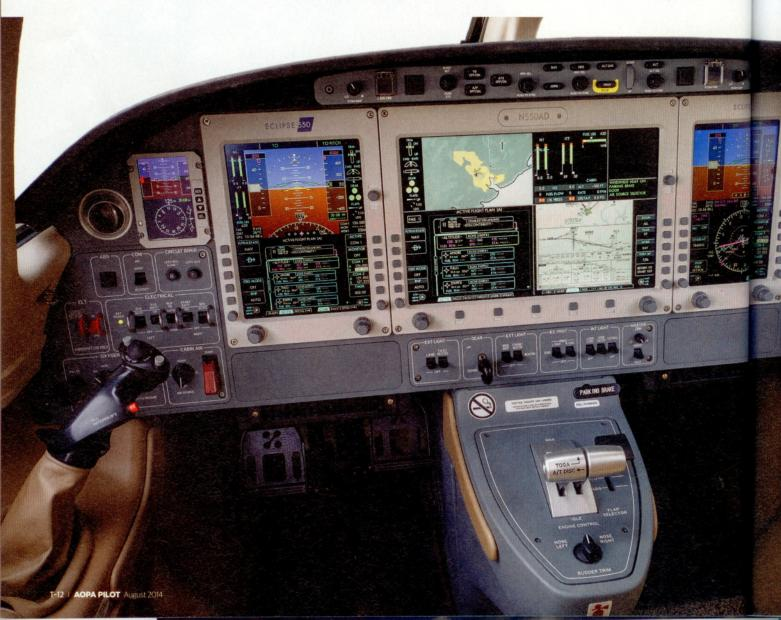
an airplane with the systems and avionics that one would expect in a jet—and some you wouldn't expect in a light, or even a medium, jet. Most notable is the inclusion of autothrottles, which were originally envisioned for the airplane by designer Vern Raburn. In fact, every airplane produced had the servos and other gear for autothrottles installed in the center console, but the system was never fully developed.
